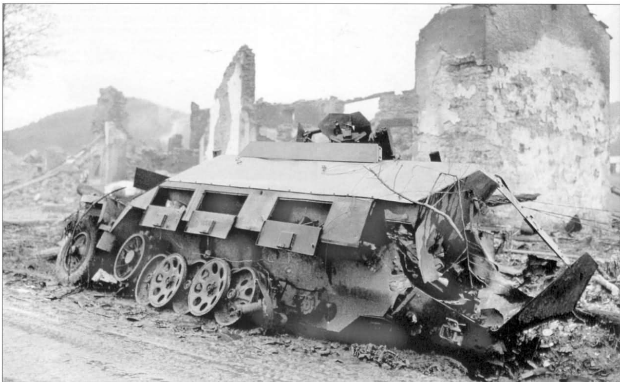
A Fliegerabwehr Schützenpanzerwagen (2cm MG151 Drilling) Sd.Kfz. 251/21 Ausf. D lies destroyed along the side of a road. The vehicle was torn by high explosives, which have ripped and ruptured the body's armor. The tracks have been completely blown away, the rubber on the road wheels has been blown away, and the open storage lockers are devoid of contents. Note the smaller shield above the mount which protected the gunner and his telescopic sight. There were two different gun shield arrangements, as well as variations of the short armor panels along the hull's upper edges.
