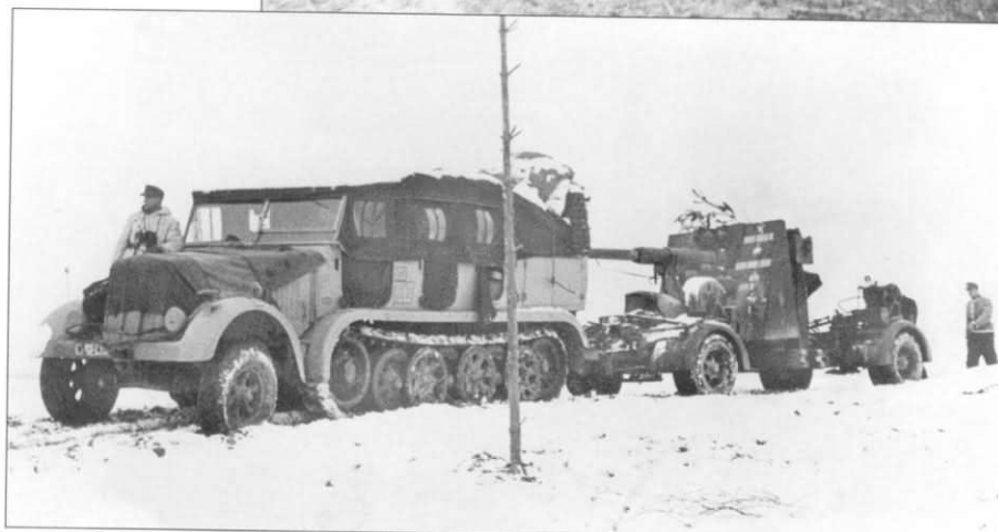
A relatively fresh-looking Sd.Kfz. 7 pulls a rather scruffy veteran 8.8cm FlaK 36/37 on a Sd.Ah. 203 limber. Note the score on the gun's shield and the R.A. 9 sectional gun tube. The tractor is in the base color of Dunkelgelb RAL 7028, and also sports a shipping stencil between the first and second rows of seats. The boarding handles are cut into the vehicle's sides while the Notek lamp is mounted on the fender over the front wheel.
