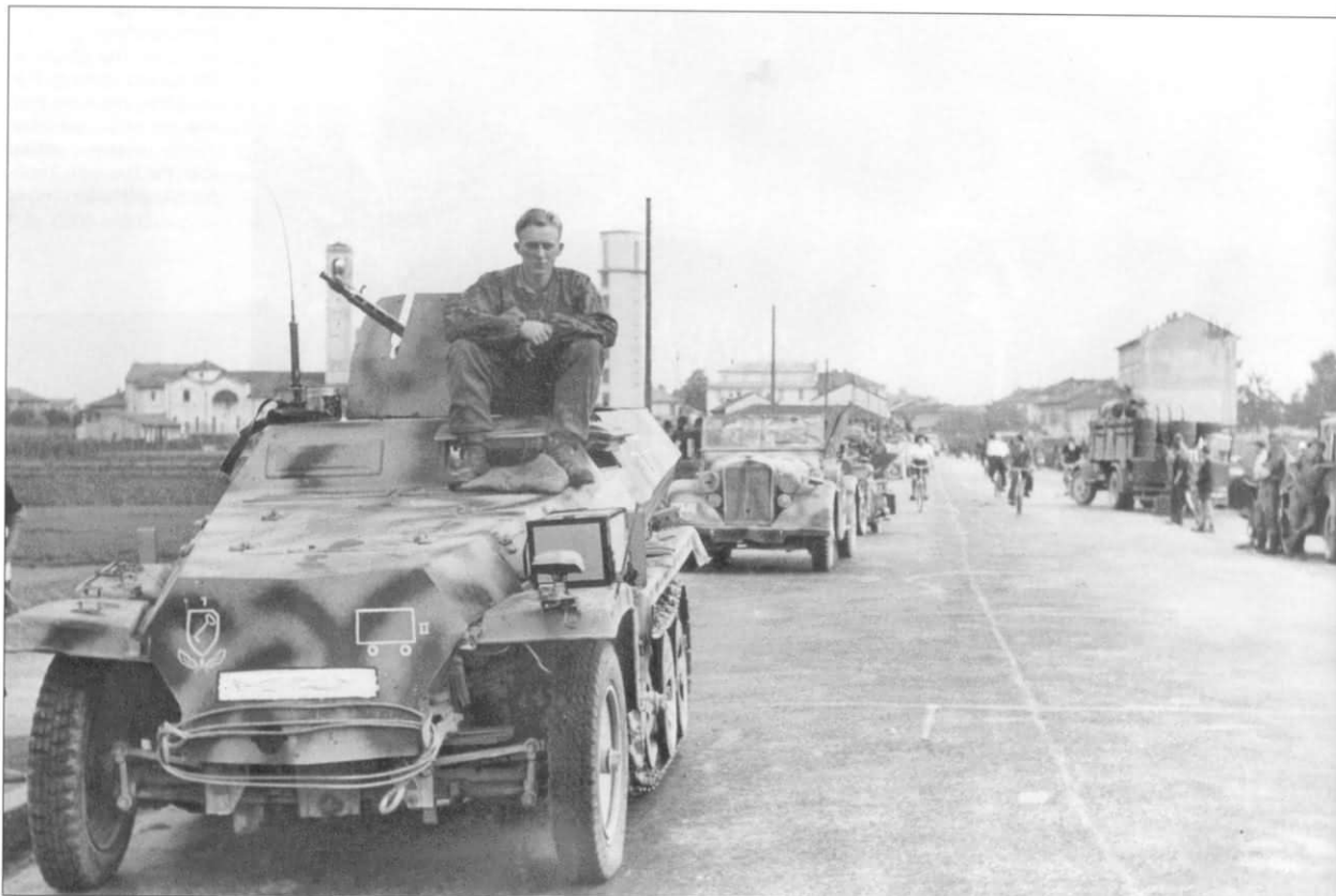
This Sd.Kfz. 250/1 of 1.SS-Panzer-Division "Leibstandarte Adolf Hitler" completely lacks its conventional headlamps, making do with only the Netek blackout-driving lamp. The tactical sign on this camouflage-painted vehicle indicates that it belongs to a rifle platoon from either SS-Panzer Grenadier Regiment 1 or 2. Note also the extended-height gun shield mounting an MG42 and the strange-looking antenna-like device next to the MG shield.
