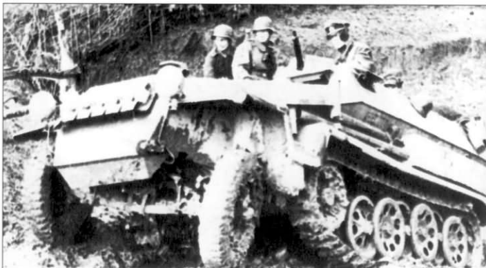
As it negotiates some rough terrain, we are afforded a view under the nose of a very muddy Schützenpanzerwagen. This Ausf. C has its head-lamps mounted as well as a Notek black-out driving lamp; note the electrical conduit for the lamps, just behind the front armor plate. Helmets and other personal gear hang on the superstructure sides, a common practice as internal space within these vehicles was always at a premium.
