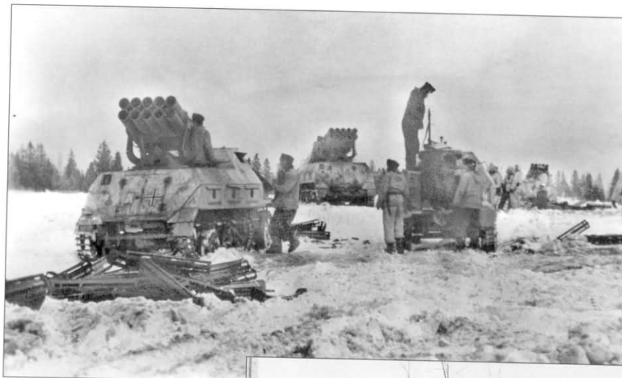
Several Panzerwerfer and a lone Munitionskraftwagen, photographed during a re-supply evolution. Note that the launch tubes of the near Panzerwerfer are trained in a direction that differs from the other vehicles so as to allow easy access to the roof hatches. There is also a heap of packing frames for the 15cm rockets in the left foreground as well as elsewhere in this photo.
