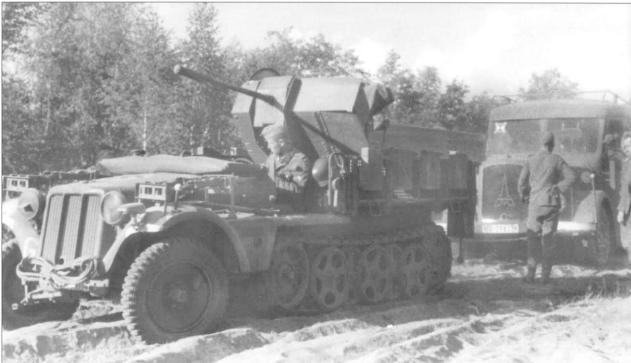
Another Sd.Kfz. 10/4 with 2cm FlaK 30 pulls a Magirus truck (note the logo on the face of the radiator) along a track. The sides of the vehicle are folded up, the road wheels are of the first pattern and the rifle racks are not covered. There is a Notek lamp fitted and the driver's windshield is encased in canvas to prevent its reflection from attracting the attention of the enemy.
