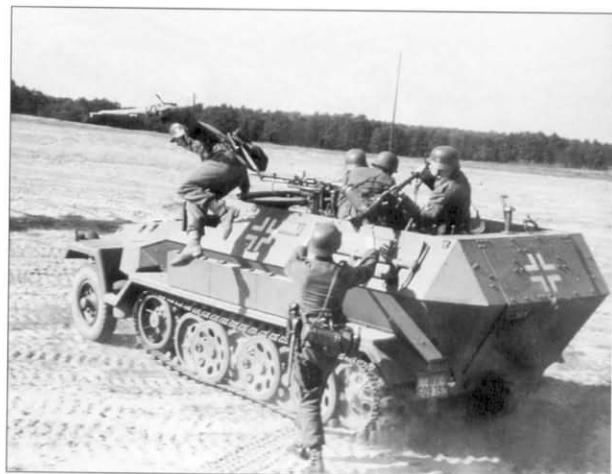
This Sd.Kfz. 251/1 Ausf. A also appears to be involved in a training exercise. It is identified as an Ausf. A by the three view-ports on the upper sides of the superstructure armor plates. Note that the forward MG34 is attached to the sustained-fire mount, while the second MG34 is being handed over the side of the half-track to a dismounted soldier; the radio antenna is also mounted in the usual spot on the right-hand forward side of the superstructure. The vehicle is plainly marked with white outline Balkenkreuze, as well as Wehrmacht Heeres license plates.
