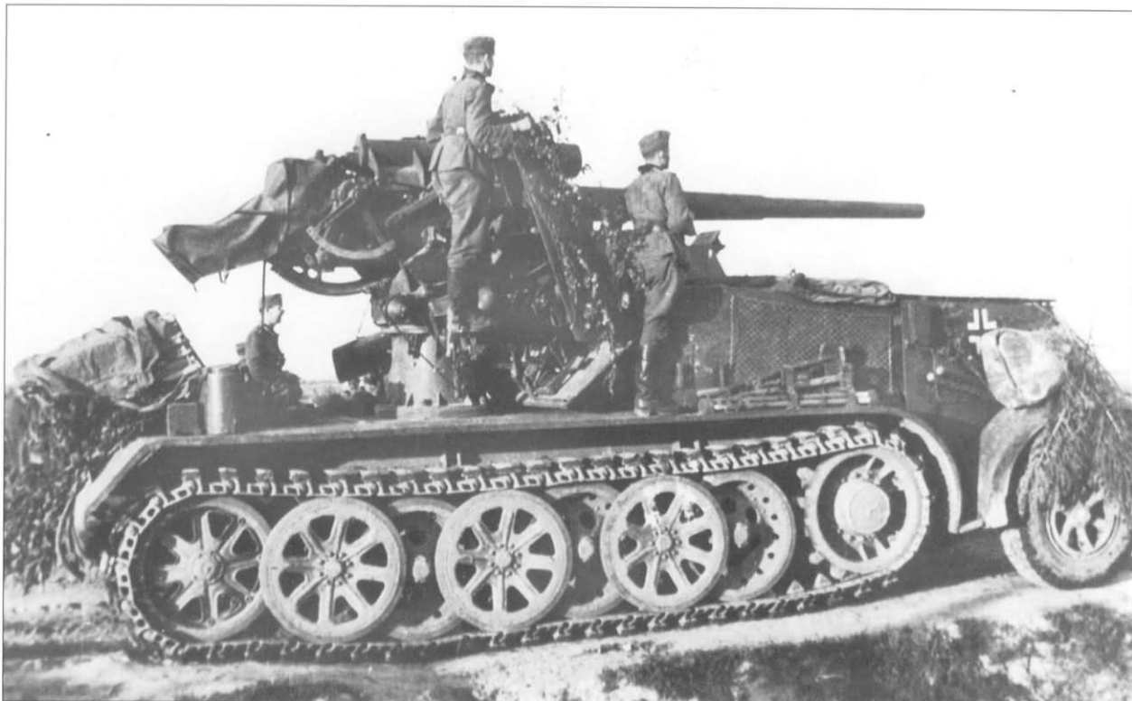
An intact 8.8cm FlaK 18 Sfl. Auf 12 ton Zugkraftwagen awaits an order to move. Note the cover on the 8.8cm gun's breech and the sparse vegetation used as a half-hearted attempt at camouflage. A close examination of the relationship of the rear of the gun, the pedestal and the vehicle's floor, will reveal one of the fallacies surrounding this gun: that it was a dual-purpose anti-aircraft and anti-tank vehicle. The gun could only elevate +15-degrees, and also had limited movement in azimuth of 151-degrees left or right of the vehicle's centerline; therefore it could not engage aerial targets.
