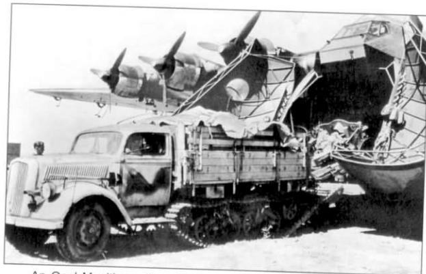
An Opel Maultier pulls a 10.5cm le.FH 18 down the nose ramp of a Messerschmitt 323 "Gigant" transport plane. The Maultier was based upon the Opel-Blitz 3-6-36S with a British-inspired Carden-Lloyd suspension system mounted in place of the dual rear wheels. It could tow a three-ton trailer or similar load, which would have enabled it to pull the le.FH 18, as seen here. The Opel Maultier was powered by a six-cylinder Opel engine, which developed 68 hp at 3000 rpm. This gave the vehicle a top speed on roads of 24 mph and a range of 100 miles.
