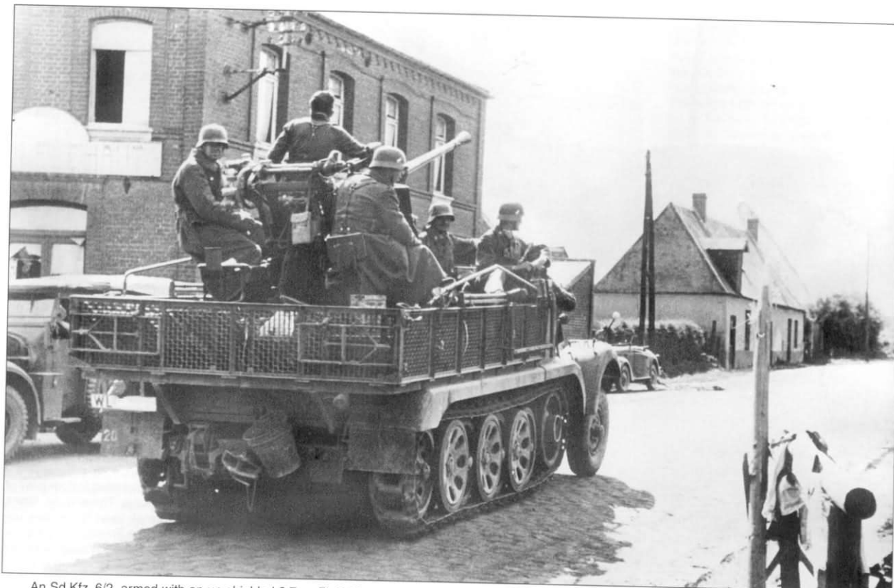
An Sd.Kfz. 6/2, armed with an un-shielded 3.7cm FlaK 36 negotiates a cobblestone road on its way to the front. This is a Luftwaffe-manned vehicle as evidenced by the "WL" prefix on the otherwise blank rear license plate. Less than 200 were built for the Luftwaffe, with nine issued to each Flakbatterie. The 3.7cm FlaK 37 was a modified FlaK 36 with the addition of a gun shield. Note the gun barrel cleaning staffs stored on top of the near-side folding platform extension, as well as the bucket and other details of the rear end.
