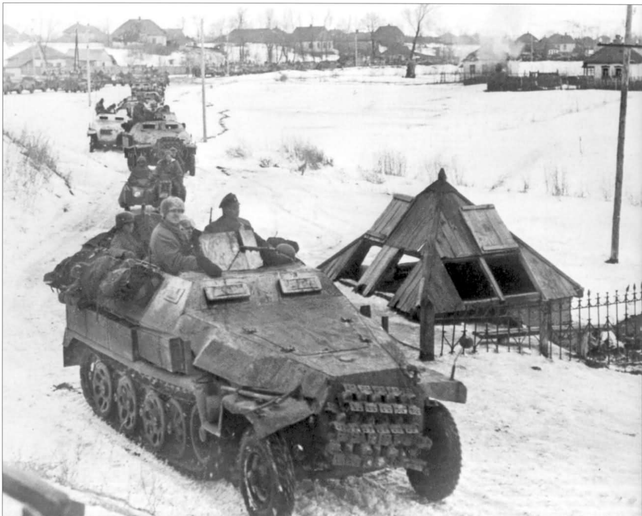
An Ausf. C whose winter white camouflage scheme is all but obliterated. Note the external stowage of the crew's personal gear, the extra box on the fender forward of the stowage lockers and the pair of spare track sections hanging on the nose plate.
