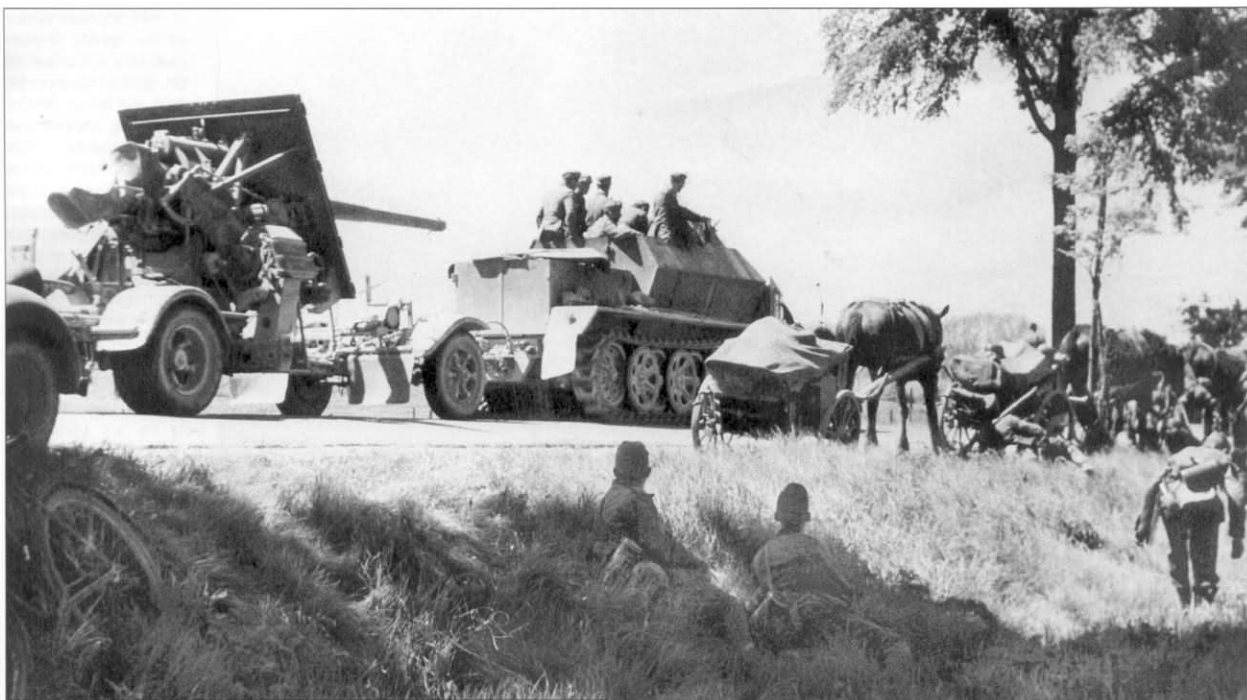
A Sd.Kfz. 7 with an armored body ("Gepanzerte 8 ton Zugkraftwagen") pulls a highly modified 8.8cm FlaK 18 on a Sd.Ah. 201 limber. Note the shield configuration, and the very unusual shape of the stabilizing outriggers. These could firmly contact the ground to stabilize the mount while the gun was still on the wheeled carriage. The combination depicted served with Panzer-Jäger-Abteilung 525, 560 and 605, during the French Campaign in 1940.
