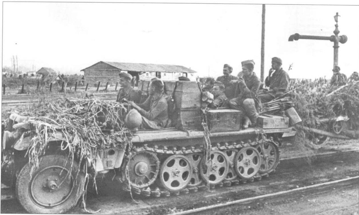
An Sd.Kfz. 10 pulls a piece of ordnance along a road adjacent to a rail line. Note the non-standard wooden structure behind the driver and the pattern of the cut-outs on the road wheels. The foliage camouflage makes it impossible to tell if the gun is a 5cm PaK 38 or a 7.5cm PaK 40, a fairly typical load. However, neither type has a hand-wheel on the right side of the mount (as seen here), nor does the PaK 97/38.
