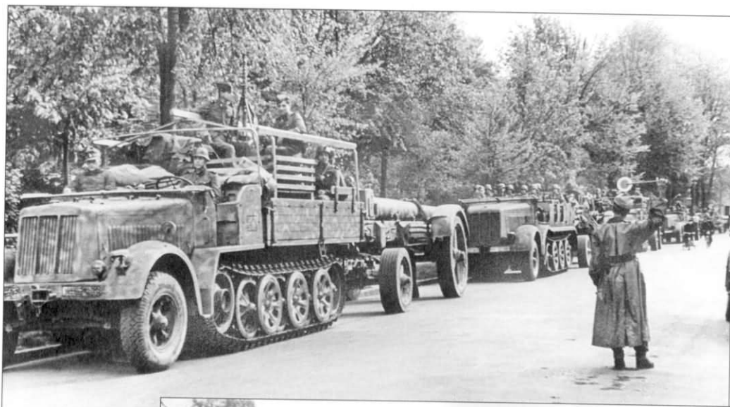
A late-war variant of the Sd.Kfz. 7 pulls part of a 17cm s.K 18 or 21cm Mörser 18, followed by an Sd.Kfz. 8, pulling another part of the ordnance. This vehicle features a wooden load-bed and a mottled camouflage. Strictly speaking, this tractor was not rated for the load it is towing.
