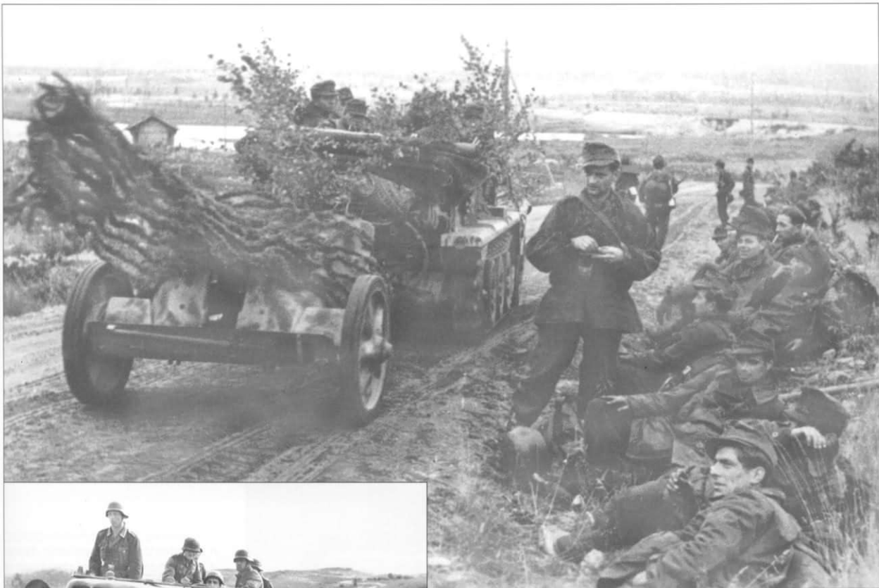
A well camouflaged Sd.Kfz. 10 pulls a 5cm PaK 38 past a tired group of "Landers". The PaK 38 can be identified at this angle by the way the lower lateral shields are interrupted by the main curved shield. The Sd.Kfz. 10, from the D7 chassis onwards, was powered by a Maybach HL42 TRKM 6-cylinder gasoline engine that developed 100 horsepower at 2800 RPM. This gave it a top speed of 40 mph, and a range on roads of 217 miles.
