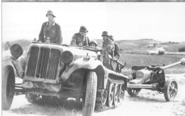
This Sd.Kfz. 10 has a camouflage scheme consisting of a lighter color brushed on in short strokes over its base paint, as can be seen below the radiator grill. Note the empty Notek lamp mount and the unusually uncluttered appearance of the tractor. The gun is a 7.5cm PaK 40, which can be identified by the shield configuration as well as the wheels with eight spokes. Modelers should note that the PaK has covers on the breech and the muzzle brake.
