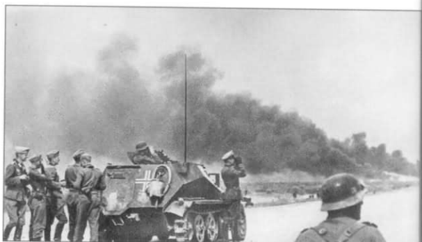
While the fires of war rage in the background, this group of Germans observes the battlefield. This vehicle is identified as a Sd.Kfz. 253 by the antenna mount, the antenna storage trough and the shape of the hatch next to the crewman.
