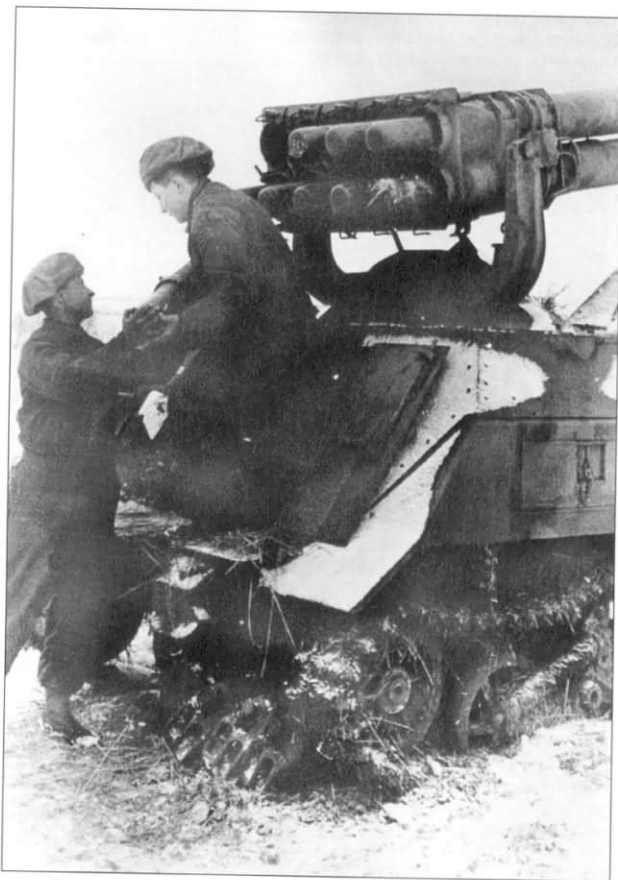
A close-up of a crewman loading the 15cm launch tubes. Note how the two rockets already loaded have their ends held in place with a small levered device. Also note the small exhaust nozzles placed around the rocket body, as well as the "U"-shaped conduits along the top and bottom edge of the launch tube assembly, which connected the rockets to the electrical firing system.
