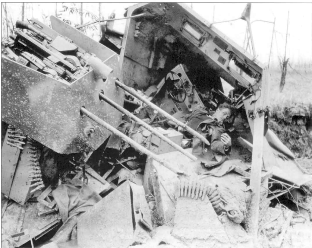
A Fliegerabwehr Schützenpanzerwagen (2cm MG151 Drilling) Sd.Kfz. 251/21 Ausf. D lies destroyed along the side of a road. The vehicle was torn by high explosives, which have ripped and ruptured the body's armor. The tracks have been completely blown away, the rubber on the road wheels has been blown away, and the open storage lockers are devoid of contents. Note the smaller shield above the mount which protected the gunner and his telescopic sight. There were two different gun shield arrangements, as well as variations of the short armor panels along the hull's upper edges.
