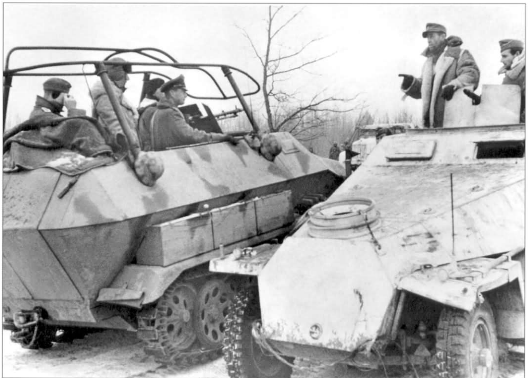
A pair of German officers observes some far-off event from the top of their Sd.Kfz. 251/3 Ausf. C. Note that one of the engine deck access hatches is open, the welded-style Ausf. C-type cowl over the air intakes (a cast version existed) and the MG34 on the shielded mount. The pennant in the foreground indicates that this mittlerer Funkpanzerwagen belongs to a Panzer division's headquarters.
