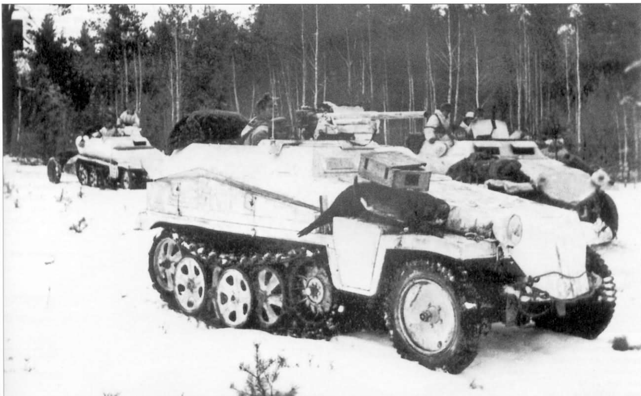
Platoon commanders had instant light anti-tank support in the form of their command vehicles fitted with a 3.7cm PaK 36. In this case, the gun's shield is of the abbreviated sandwich-armor variety, on this white-painted Sd.Kfz. 250/10 Ausf. A.
