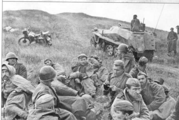
Captured Red Army troops take their rest in the lee of a hill, guarded by a Sd.Kfz. 253. Just visible on the forward portion of the '253's roof is the rotating cupola, which mounted a S.F. scissors periscope. The crewman is standing in the square opening of the rear hatch.
