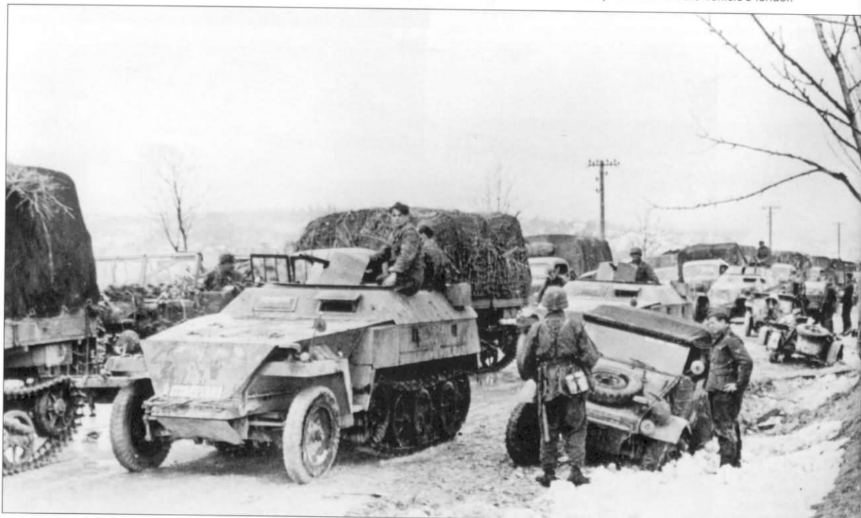
A column of SS vehicles on a snow-bound road, pass a Volkswagen Type 82 Kübelwagen. The first half-track is a Sd.Kfz. 250/1 Ausf. B, the second appears to be a Sd.Kfz. 250/3 leichter Funkpanzerwagen radio vehicle (note the canvas covers on the antenna bases), while the third one is a Sd.Kfz. 250/9 Ausf. B, mounting a 2cm auto-cannon. To the left of the column of '250s, is a pair of Maultier cargo half-tracks, with the first towing an unidentified load. The lead '250 has a faint Tac number "23" on the front plate. Further down the road are a VW Type 166 "Schwimmwagen" and a heavy motorcycle with sidecar.
