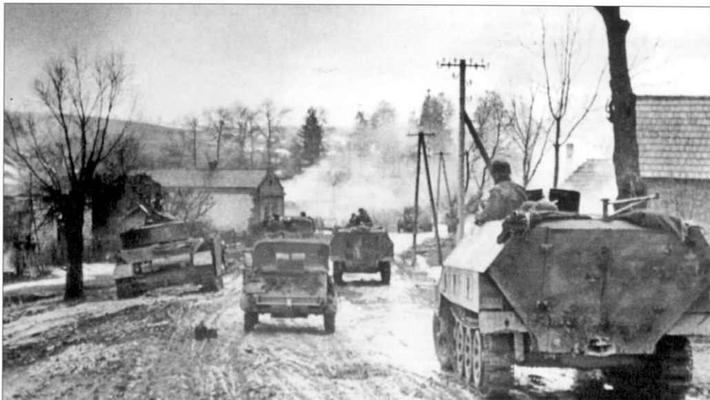
A group of German panzers, m.SPWs and a lone VW Kübelwagen advances towards the enemy, again illustrating the actual practice of combined-arms operations. The Pz.Kpfw. IV is probably an Ausf. H as can be seen by the small, square muffler for the turret traverse motor seen on the left side of the rear plate.
