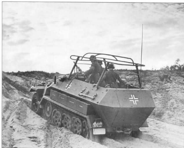
An Sd.Kfz. 251/3 Ausf. B passes through a sandy area, while negotiating an incline. This vehicle is unique in having four (normally, only three were fitted) stowage lockers on the rear side, all of which have stenciled information on them. There is a rod antenna on the rear superstructure edge, as well as the usual "Rahmanantenna" (frame antenna). The forward machine gun lacks a shield and the vehicle is fitted with the Notek black-out driving system.
