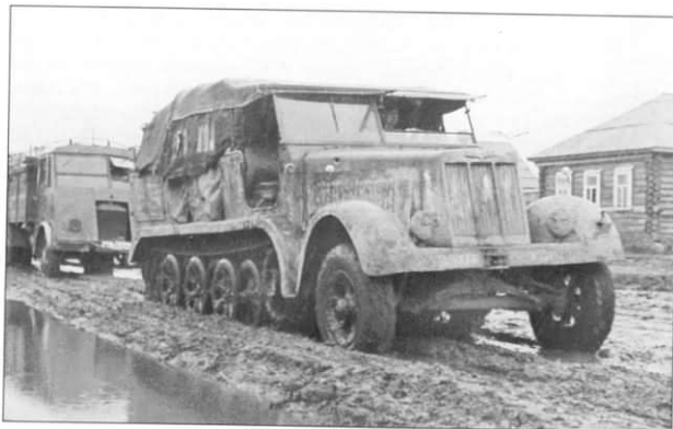
Doing what it does best, an Sd.Kfz. 7 tows a lorry through the mud. Note that this vehicle has a different position for the mount of the Notek black-out driving lamp, although the lamp itself is missing. Also note how the driver's wind-shield has a separate fold-out panel, which is seen here in the raised position.
