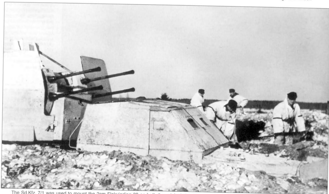
The Sd.Kfz. 7/1 was used to mount the 2cm Flakvierling 38 on both the original chassis, or, as seen here, on a partially armored chassis that had a shield in front of the radiator and an enclosed (open to the rear) driver's cabin. This white-painted vehicle has also been dug in to the frozen ground while it awaits the next enemy onslaught. This dual-purpose mount was devastating against infantry in the open and was also much feared by the crewmen of low-level ground-attack aircraft.
