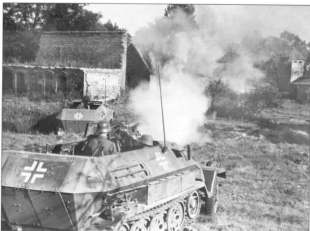
A Sd.Kfz. 251/10 Ausf. B is photographed at the moment of firing its 3.7cm PaK 36. The gun has a partial shield on its left side to protect the gunner while he mans the sights. This dusty vehicle has a rod antenna mounted in the more-or-less standard location.
