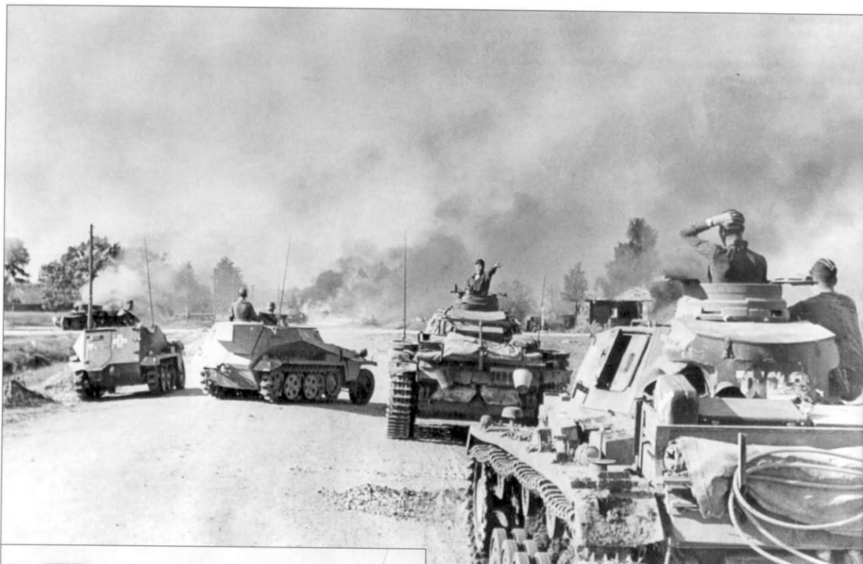
Dubbed the "Leichte Gepanzerte Beobachtungskraftwagen", a pair of Sd.Kfz. 253s occupy the middle of a road accompanied by a pair of Pz.Kpfw. IIIs. Note the large stowage box on the center '253's rear plate and the opened semi-circular hatch on the roof; the latter feature positively identifies this as a '253.
