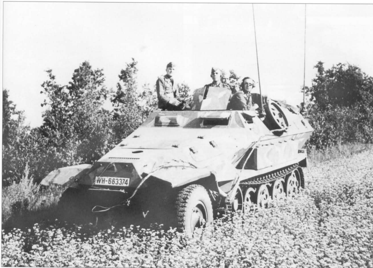
The pair of antenna bases identifies this half-track as a probable Sd.Kfz. 251/3, while the lack of extra view-ports identify it as an Ausf. B chassis. There were several variations of the basic version, two of which were used by Luftwaffe personnel for coordination with air assets. The attitude of the crew as they appear to gaze skywards may also indicate that cooperation with nearby aircraft is taking place. Note the tow cable and spare road wheel stored on the vehicles rear side, the Wehrmacht Heeres license plate and the hard-edge camouflage visible in certain areas where bright light has not washed out the original print.
