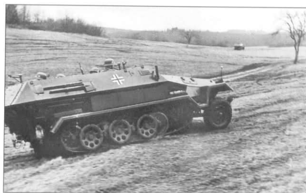
A Sd.Kfz. 251/1 Ausf. B moves up a slight incline, with its mate in the far background. Note the anti-aircraft-style machine gun mounts both fore and aft, the two different styles of shovel stored on the superstructure, and the neat appearance of the vehicle.
