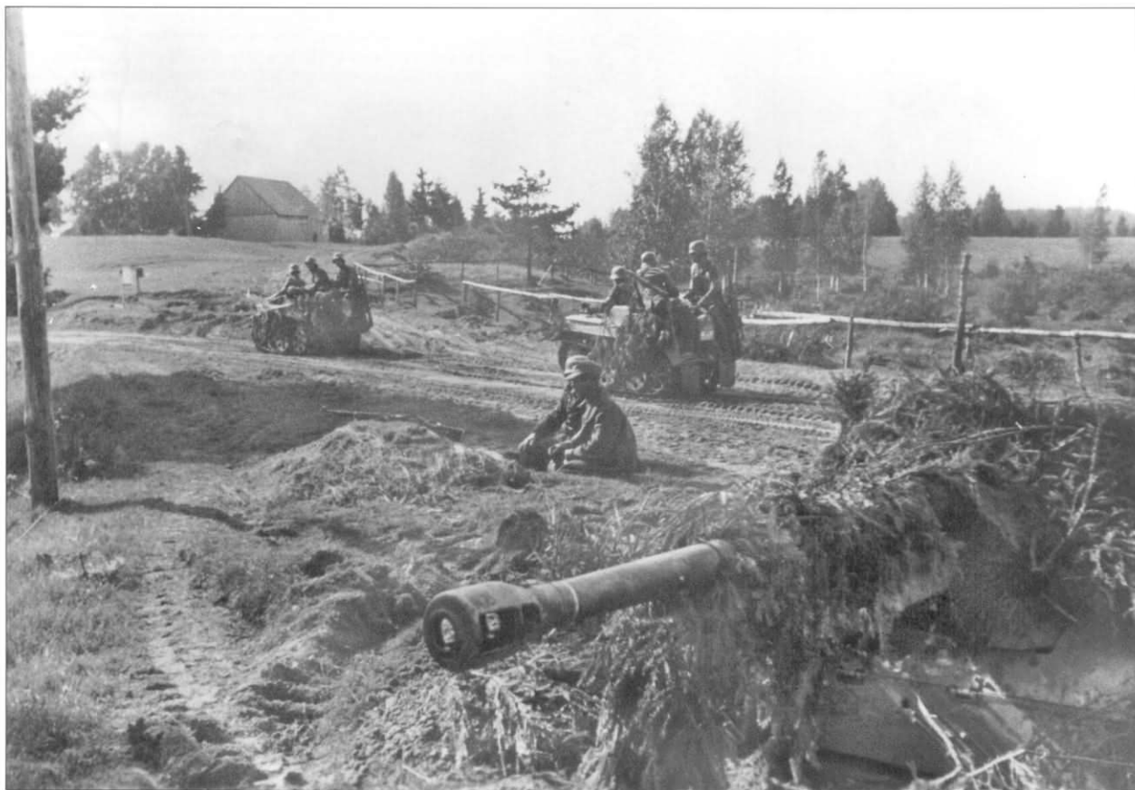
A mini-convoy of Kettenkrads passes a well-sited and camouflaged 5cm PaK 38 anti-tank gun. Note how the Kettenkrads are over-loaded with passengers, and that they move in a "tactical sense", i.e., too slow to raise a tell-tale cloud of dust, which would alert an observant enemy to their location.
