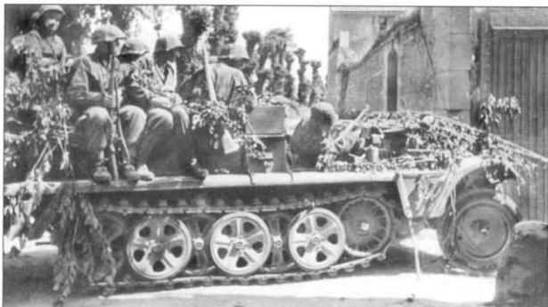
This well-camouflaged Sd.Kfz. 10 has the second pattern road wheels and carries an infantry section garbed in camouflage clothing. Note also that there is a structure behind the driver's compartment similar to that seen in an earlier photograph.
