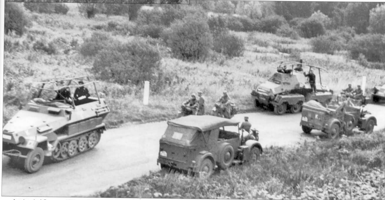
A column of German AFVs and motorcycles pause across the road from a pair of Kfz. 15 medium cross-country cars. A Sd.Kfz. 251/3 Ausf. A is followed by a Panzerfunkwagen Sd.Kfz. 263 (8 Rad) and a four-wheeled armored car of indeterminate type. Several vehicles have a white "K" applied, which denotes their attachment to Panzergruppe von Kleist. Note that the '251/3 has a full set of three stowage lockers. No vehicle shown here is equipped with a Notek lamp, which along with the white "K", identifies this photograph as having been taken during the French Campaign of 1940.
