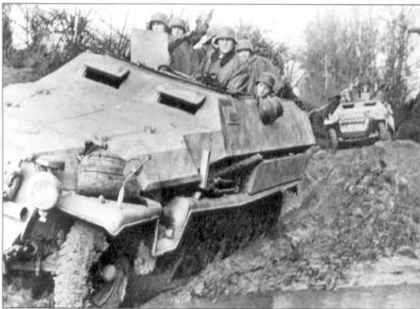
Yet another muddy, scruffy Ausf. C fords another small water obstacle. Of note is the unusual configuration of the cowl that covered the engine air intakes on the near-side of the half-track. This vehicle has a full complement of head-lamps, as well as a Notek lamp, while it mounts an MG42 behind the forward shield.
