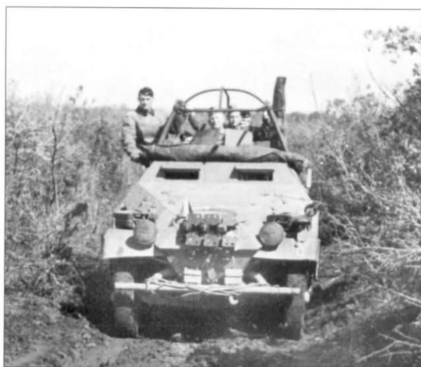
This Sd.Kfz. 251/6 Ausf. B moves along a path through a brushy area. There is an 8-meter "Kurbelmast" (telescoping antenna mast) covered in canvas protruding through the "Rahmanantenna" (frame antenna). Note also the Notek lamp mounted on the fender, spare track sections on the bow and the canvas-covered conventional head-lamps.
