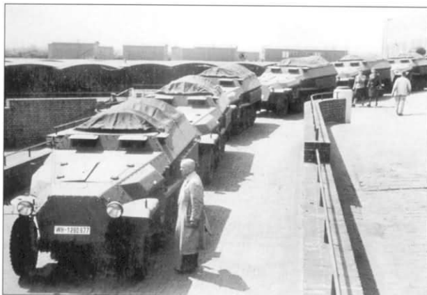
A line of Ausf. Cs leave the factory. These are the riveted hulls only seen on some Ausf. Cs. Each has its troop compartment covered by a tarp stretched over the internal half-hoops. The conventional head-lamps are without any hoods, there are no tools seen, the forward gun shields are not fitted and the Netek black-out driving system is also absent.
