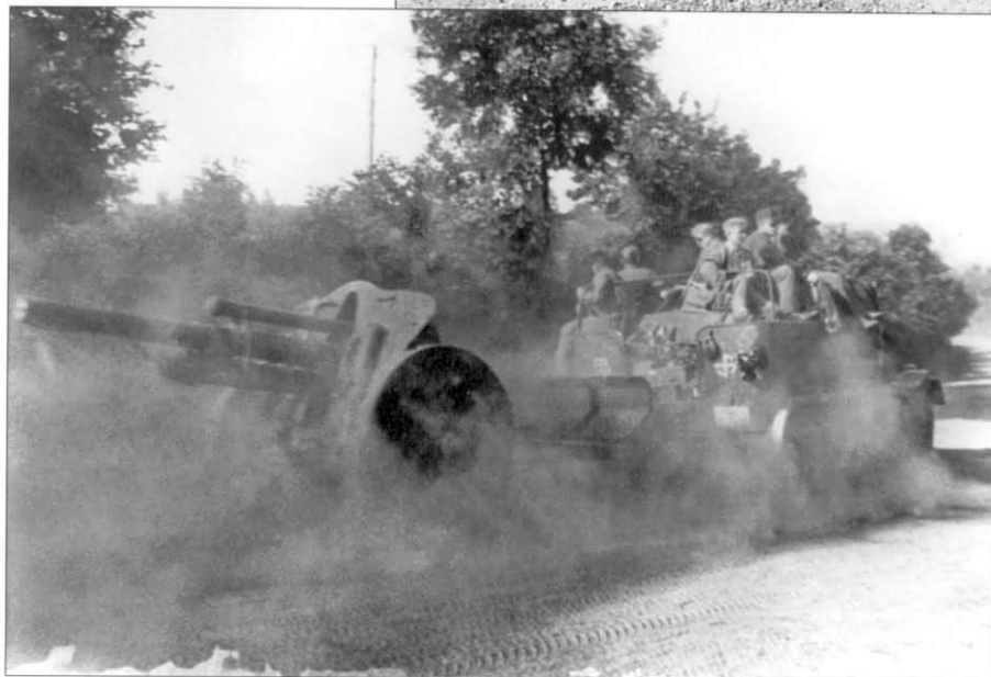
Sd.Kfz. 11 belonging to SS-Division "Wiking" throws up a cloud of dust as it speeds along pulling a 10.5cm le.FH 18 from SS-Artillerie Regiment 5. Power was provided by the same 6-cylinder Maybach HL 42 TUKRM gasoline engine as used on the Sd.Kfz. 10, which produced 100 horsepower at 2800 rpm. This drove the vehicle at 33mph on roads to a range of 172 miles. Combat weight with 9 men on board was 7.2 tons while 3 tons could be towed. The vehicle was 18.3 feet long, 6.6 feet wide and 7.1 feet high, overall.
