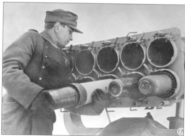
A close-up of a crewman loading the 15cm launch tubes. Note how the two rockets already loaded have their ends held in place with a small levered device. Also note the small exhaust nozzles placed around the rocket body, as well as the "U"-shaped conduits along the top and bottom edge of the launch tube assembly, which connected the rockets to the electrical firing system.
