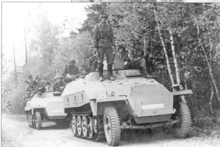
The other main distinguishing feature of the Ausf. D hull is the configuration of the storage lockers, which are continuous and integral with the lower fenders. All previous versions had separate lockers mounted on various locations on the fenders. Note also that this m.SPW has the earlier Notek black-out driving lamp and is painted in the base color of Dunkelgelb RAL 7028.
