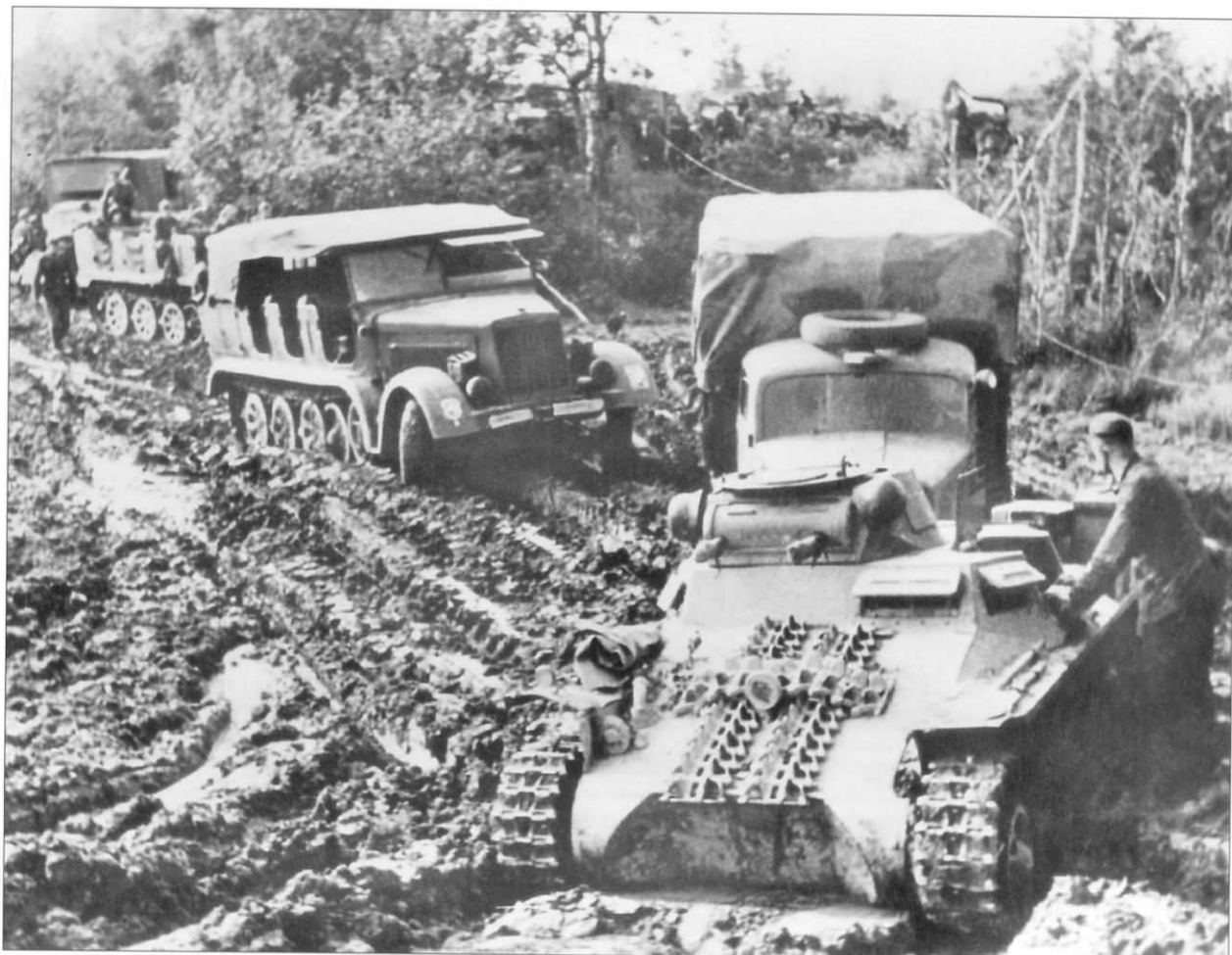
A Sd.Kfz. 7 is preceded on a muddy track by a Pz.Kpfw. I and a lorry, with the remainder of a convoy lined up behind it. The KMm 11 version of this vehicle (shown) was powered by a six-cylinder Maybach HL 62 TUK (or HL 64 TR), which developed 140 hp at 2600 rpm. This gave the vehicle a maximum road speed of 31 mph and a range of 156 miles.
