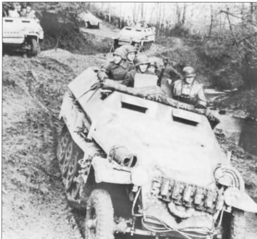
A group of Ausf. Cs negotiates a rather rough ravine running alongside a small creek. As was the case in the previous photo, a length of spare track is stored on the front plate. The first vehicle mounts a Notek lamp on the front fender and carries an MG42 behind the front shield.
