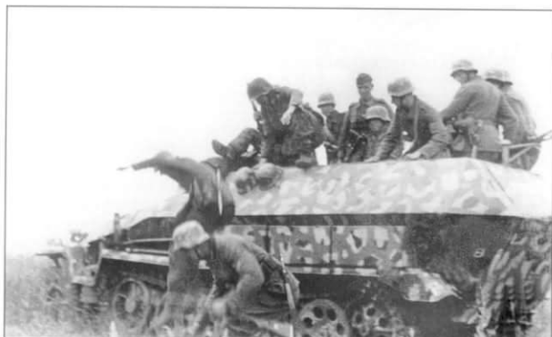
This fully-loaded Sd.Kfz. 251/1 Ausf. C disgorges its section of Panzergrenadiers. It is painted in a very unique hard-edged camouflage scheme featuring at least three colors applied in a very tight dapple pattern. The vehicle can be easily identified as an Ausf. C by the shape of the cowls on the sides of the engine compartment. Other identifying features are the location of the storage lockers and the shape of the fender both at the rear end and where it bends upwards in front of the forward locker.
