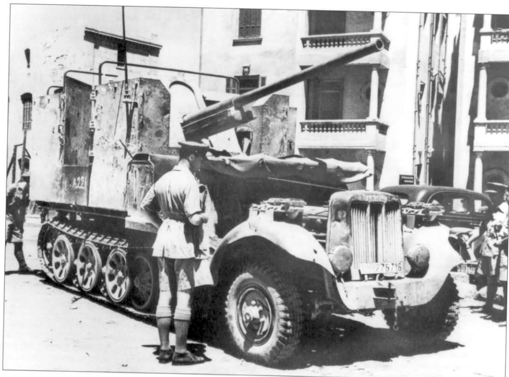
An Sd.Kfz. 6/2, armed with an un-shielded 3.7cm FlaK 36 negotiates a cobblestone road on its way to the front. This is a Luftwaffe-manned vehicle as evidenced by the "WL" prefix on the otherwise blank rear license plate. Less than 200 were built for the Luftwaffe, with nine issued to each Flakbatterie. The 3.7cm FlaK 37 was a modified FlaK 36 with the addition of a gun shield. Note the gun barrel cleaning staffs stored on top of the near-side folding platform extension, as well as the bucket and other details of the rear end.
