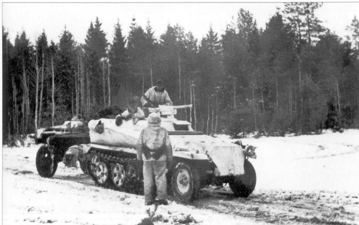
Belonging to the same group as the previous Sd.Kfz. 250/10 Ausf. A, this /10 tows a trailer of undetermined type. It is also covered in white paint for concealment in the snow, and has the abbreviated sandwich-armor shields attached to the gunner's side of its 3.7cm PaK 36.
